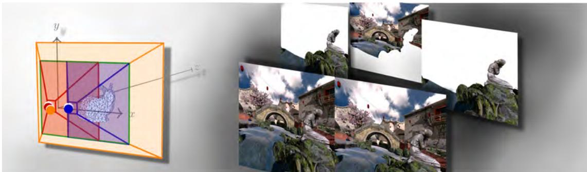
Figure 1: Visualization of the camera setup and the assembly of a hybrid stereoscopic image pair using only one image to serve for the far region (beyond 3m) of both stereo views.
